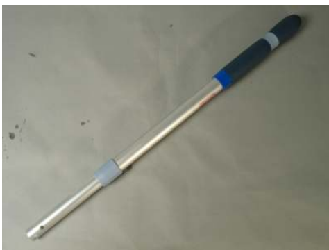
Photo 1: Telescopic Handle frame after 80 cycles
