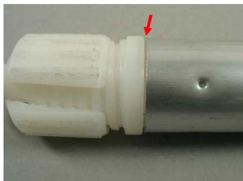
Photo 2: Inner screw becomes a bit loosen
